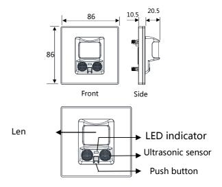
LED indicator: Red for PIR, Green for Ultrasonic, Orange for both PIR and ultrasonic
