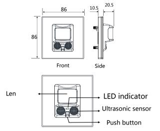
LED indicator: Red for PIR, Green for Ultrasonic, Orange for both PIR and ultrasonic
