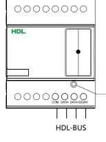
Flicker when the module is working fine. Keep pressing the indicator for 3 seconds, it turns to red color, then it is read and the address of the module can be modified in the HDL Bus Pro set up software.
