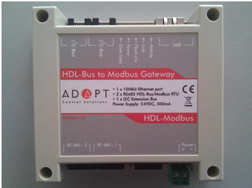
By HDL-Bus to Modbus Gateway you can integrate any HDL-Bus control system into your BMS, SCADA, PLC ... “talking” Modbus.
