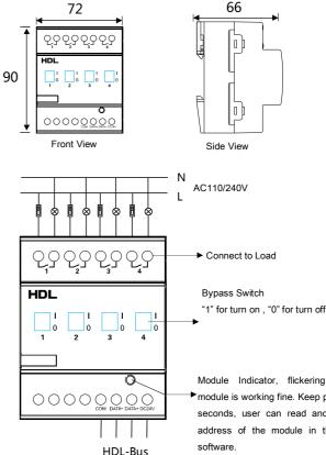
Module Indicator, flickering when the module is working fine. Keep pressing for 3 seconds, user can read and modify the address of the module in the HDL-Bus software.
