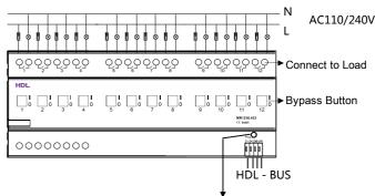
Indicator of module & easy programming button, flicker when the module is working fine, keeping press the indicator for 3s, it turns red color, The address of the module can be read and modified in the HDL-BUS Pro software.
