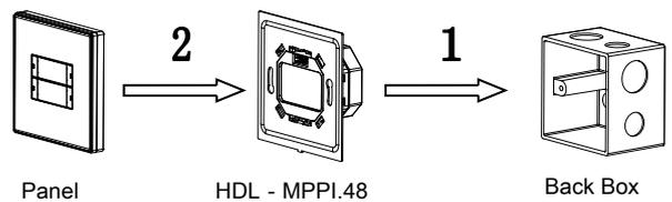
**Remove Panel:** use slotted screwdriver to insert the split gap, separate the panel and power module ( MPPI.48 )
