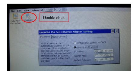
The IP address of touch screen and host PC must under the same network segment.
