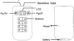
**Sensitive tube :** the LCD background light is on when there is no enough light.
