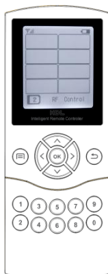
Fig. 13 RF panel interface
