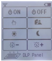
Fig. 10 Floor heating interface
